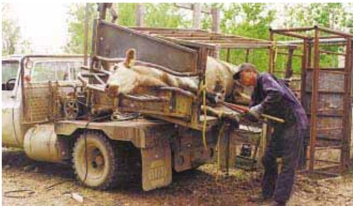
Brandl built his own trimming table and mounted it on back of his 1981 Chevy 1-ton flatbed truck. Head gate allows cows to walk through when they're finished.
