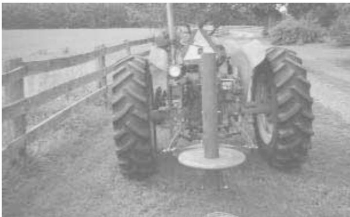
The 3-pt. mounted wire unroller is made from a piece of 4-in. dia. pipe and two 20-in. round steel plates - one bolted down and one left free to turn with the wire as the tractor goes along.
