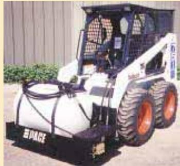
Self-contained pressure washer attaches quickly to skid loaders.
