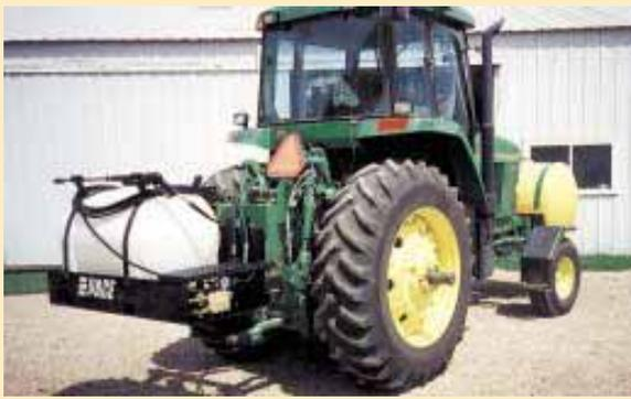
Unit also mounts on a tractor Cat. II hitch, using 3-pt. hitch adaptors that attach to the platform.
