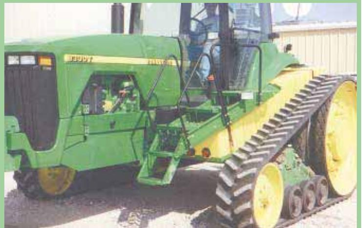
Tanks mount between tractor frame and tracks so they don't interfere with cab access and operator visibility. Each tank holds up to 260 gal. of liquid fertilizer or chemicals.
