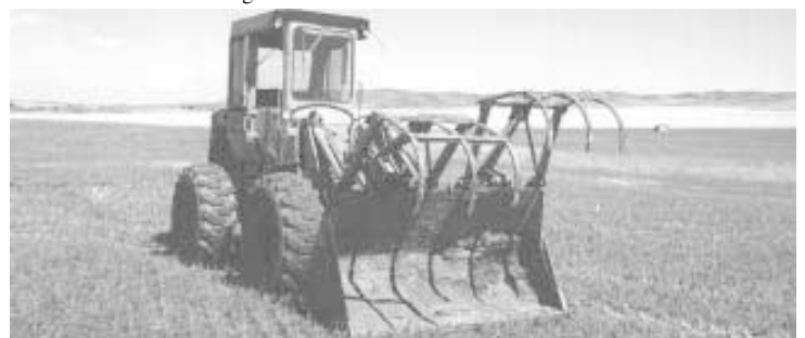
Modified payloader has two independently controlled grapple forks for fast loading.
