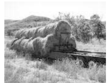
Side rails provide stability for trailer and also make a track for the push-off bar to run on.
