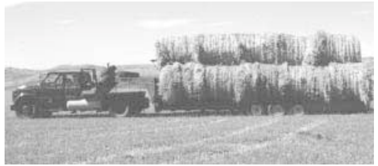
Brown's 28-ft. long bale hauler holds 15 5-ft. wide bales and 18 smaller 4-ft. bales.
