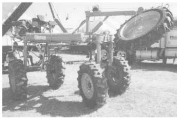
High clearance rig can go through standing corn without damaging it. Boom on front is fitted with an electric winch that can be used to lift tires, engines, or other parts.
