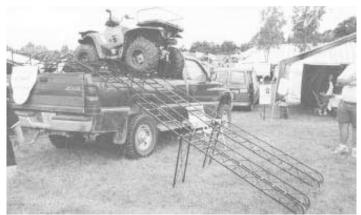
Ramp system consists of four separate steel arches that mount in pickup bed. Side ramps run from ground up to pickup.
