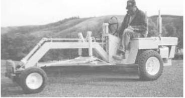
Fun-to-drive road grader is 6 1/2 ft. wide and 11 ft. long. It's powered by a 23 hp Kohler engine and is painted Caterpillar yellow.
