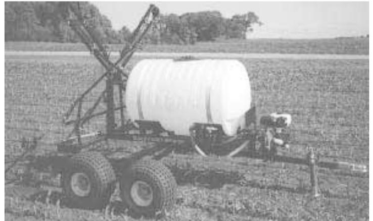
“Quality Built Sprayer” mounts on four flotation tires that are adjustable on the axle to fit any row width. Wheel spacing ranges from 54 to 90 in.
