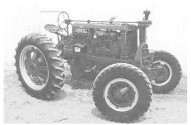
Breneman added front wheel assist to his Farmall F-20. There's a chain-driven gearbox between the clutch and tractor transmission with driveshaft leading to front axle.
