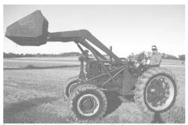
Front drive axle and traction grip tread tires are off an International Loadstar truck.
