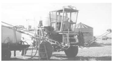
Combine's original header lift cylinders are used to raise and lower a commercial 3section boom that mounts on front.
