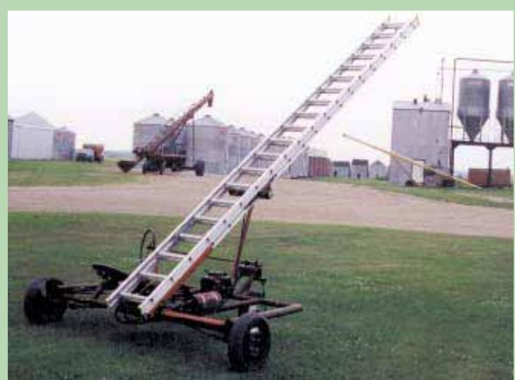
Self-propelled ladder extends up to 36 ft. It has three forward speeds and one reverse.
