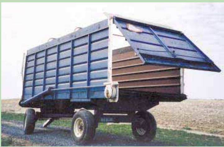
Body of wagon was turned 180 degrees on its chassis so it can unload out the rear.
