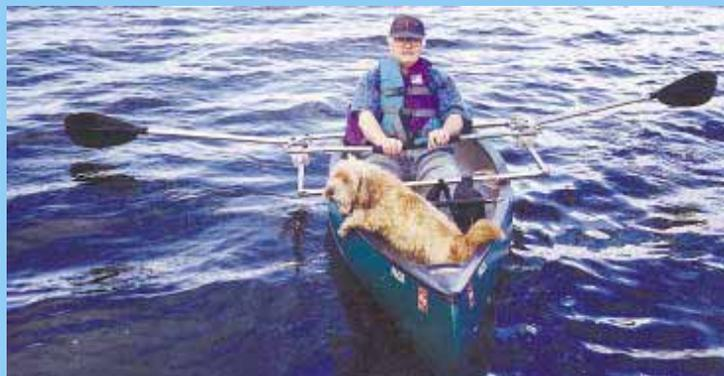
Stainless steel rowing frame simply clamps to the middle of the canoe.
