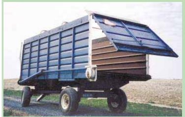
Body of wagon was turned 180 degrees on its chassis so it can unload out the rear.
