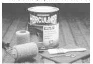
Zylene or acetone (not included). Then, scuff the surface with the pad included in the kit. Next, apply the product 1/16th in. thick per coat (apply as many coats as you desire) with the brush and rollers (included). Takes six to eight hours to set up for light-duty use; 24 hours to completely cure."
