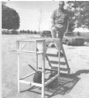
so that when he needs to move the stairs, he simply raises the bottom crossbar onto the bracket and uses a handle attached to the axle to pull them around the yard. With one hand on the top platform and one on the handle, he can easily roll the steps anywhere needed.
