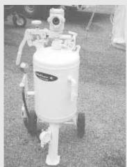
proved. It desired, the unit can etch a painted surface, so that it can be repainted without having to sand."
