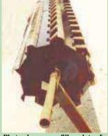
Photo shows new filler plates for Gleaner rotors.
