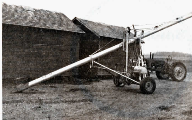
Raabel's self-propelled auger is powered by a 40 hp. gas engine. It's mounted on Deere combine chassis.
