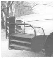
Guard slants back on both sides to protect the headlights and turn signal lights.
