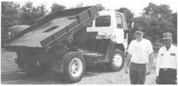
Aggert removed dump bed and hoist from a 1-ton pickup and remounted it on a modified 1988 2-ton Ford delivery truck, which he bought used.
