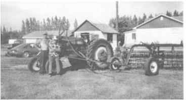
Kardynal modified hitch on an older-style, ground-driven International rake so that he can pull it alongside his Massey Harris 44 tractor.
