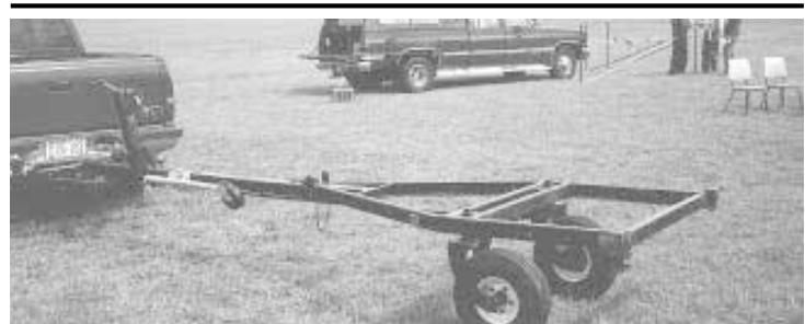
Easy-backing 15-ft. trailer is equipped with a pair of 8-in. caster wheels on back.
