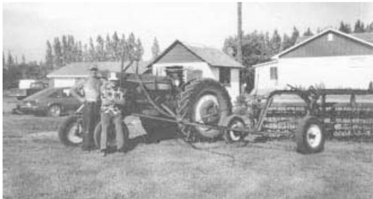
Kardynal modified hitch on an older-style, ground-driven International rake so that he can pull it alongside his Massey Harris 44 tractor.
