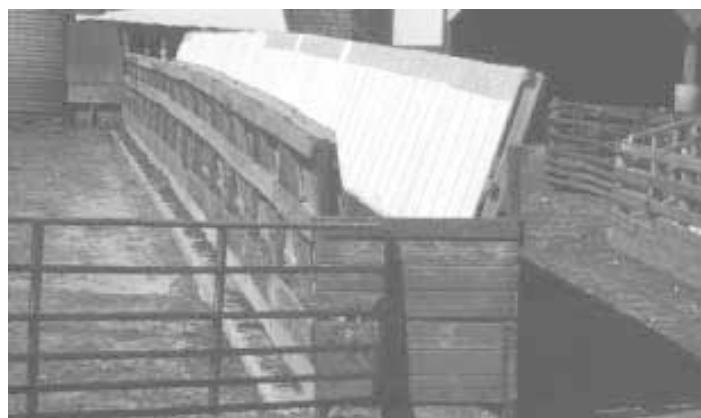
Thompson used old metal barn roofing and 2 by 4's to build a 4-ft. wide, 150-ft. long feed bunk for his feedlot. Bunk extends out from a feed room next to a pair of silos.
