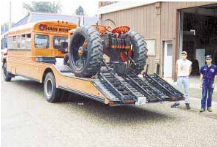
Back of bus was modified to slope downward and is fitted with three loading ramps.
