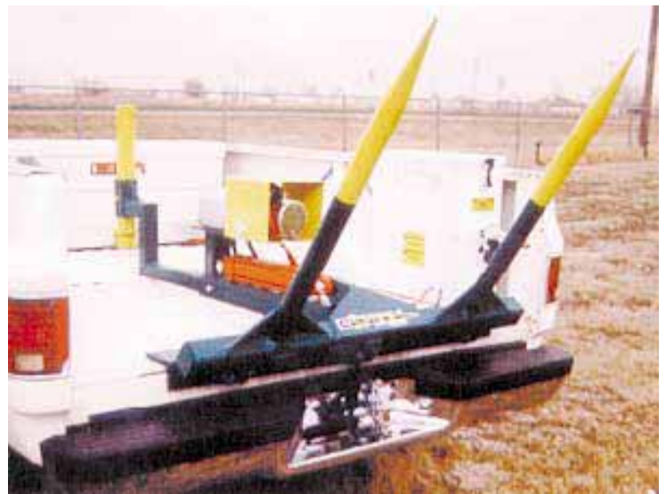
A pair of forks are raised and lowered by a 12-volt hydraulic power unit that mounts in the pickup bed.
