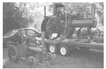
Tractor is powered by a 1936 Fairbanks Morse 3 hp water-cooled engine.
