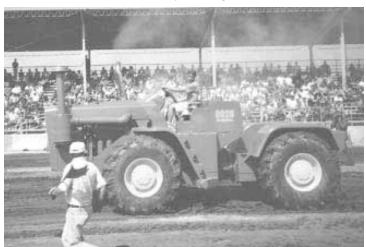
Modified for tractor pulls, this 8020 was repowered wth a Detroit 871 turbo.
