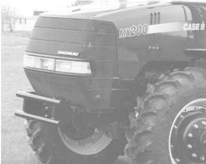
Guard, made out of hardened steel, bolts to existing holes in tractor's front end.
