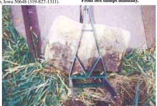
Home-built rock fork is used to dig out large rocks. You lay frame on top of rock and drive in two spikes, one on either side, then crank it up with winch.
