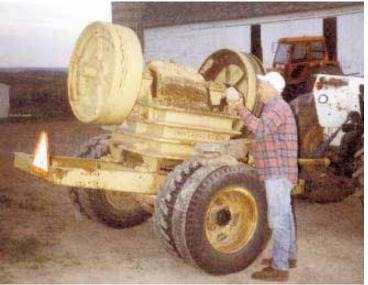
Trantham simply dumps rocks into an opening on one side of the crusher, which consists of two large jaws made from solid cast steel.
