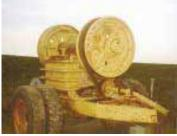
Rig is belt-driven by a 3-ft. dia. pulley that's counterbalanced by a large flywheel on back.
