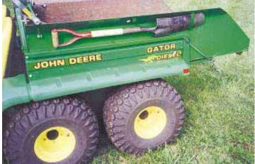
Made out of heavy 1/8-in. thick steel plate, the rock box bolts inside the Gator's existing box and can be easily removed when not needed.
