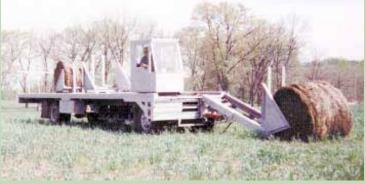
Both the cab and 11-ft. bale arm slide from one side of the deck to the other for loading.
