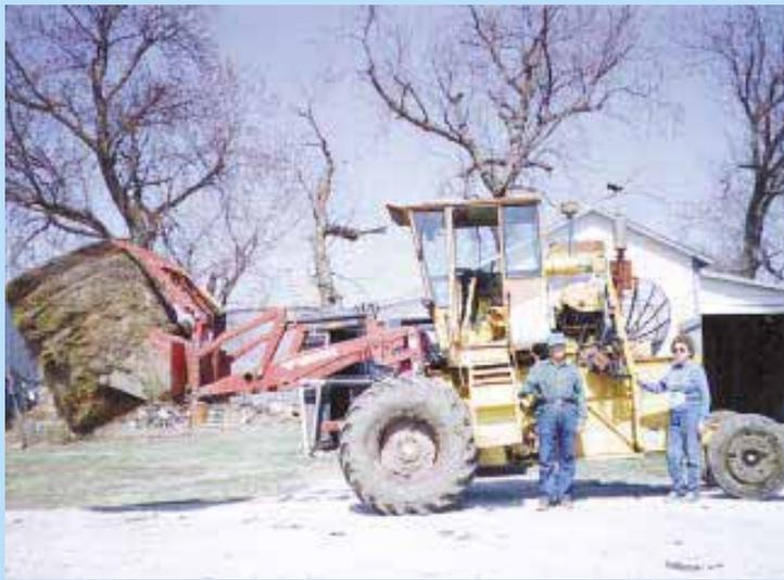
Loader tractor is built out of a late 1960's Moline combine. It's fitted with a Versatile front-end loader.
