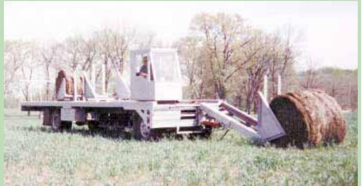
Both the cab and 11-ft. bale arm slide from one side of the deck to the other for loading.
