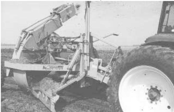
A pair of hydraulic-controlled blades adjusts to control side slope of the ditch.
