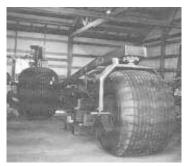
Front wheel pivots on an axle hub off a semi truck that bolts to front end of frame.
