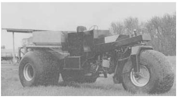
Riding on 66 by 44-in. flotation tires, the rig can be used either as a fertilizer spinner spreader or as a sprayer.
