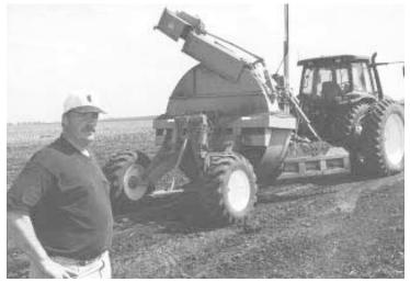
Watershed Management's ditcher has been totally reengineered into a pull-type unit.
