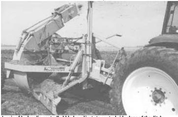
A pair of hydraulic-controlled blades adjusts to control side slope of the ditch.
