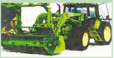
After you've used rotor to strip twine off 30 to 40 bales, you cut twine off by activating two hydraulic cylinders that move cutting teeth down onto the drum.
