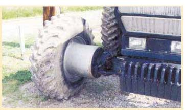
Welder Gary Hatten made "spacers" from 16-in. dia. oil field pipe. "Spacers" move front wheels out so they run in line with the outer duals on back of tractor.
