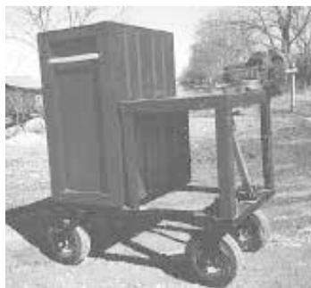
so I could mount my 5-in. vise on it. I made a hitch for the trailer out of 1 1/2-in. sq. tubing. It telescopes from 18 to 25 in. and folds underneath the table when not in use. The trailer rides on two 5/8-in. dia. steel shaft axles fitted with 3 by 10-in. pneumatic tires. I made my own front wheel swivel assembly so the rig trails my Honcho 4-WD ATV perfectly.
