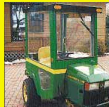
The cab mounts on the tractor with six bolts through three holes I drilled in each running board. It can be mounted and dismounted in minutes.
