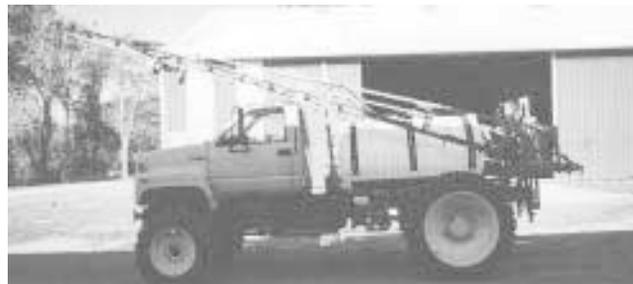
Sprayer features a 60-ft. Ag-Chem skid-mount system intended for pickups.
