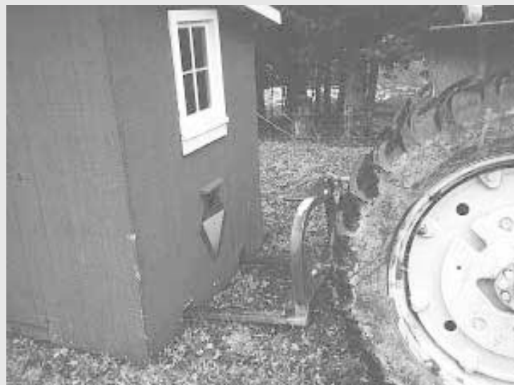
Shed is carried to the field on a pair of bale forks on Hayes' tractor's 3 pt. hitch.
