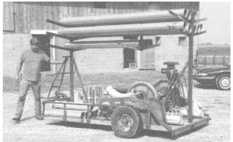
Caddy is equipped with three V-shaped racks on top that hold 24 pieces of 10 and 6-ft. pipe.
