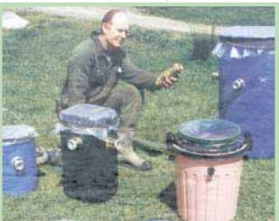
To make his prototype, Cox stuck empty beer cans into the sides of plastic buckets. Flies find their way inside through holes in the cans but then can't find their way out.
