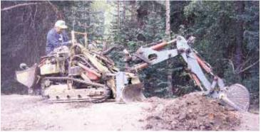
Borsky's mini dozer is just 3 ft. wide. It runs on homemade steel tracks 5 ft. long.
