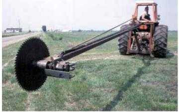
Rig uses a 26-in. dia. blade off an old buzz saw mounted on the end of a 24-ft. long boom. The Elliotts can trim limbs from 3 ft. off the ground up to 30 ft. high.
