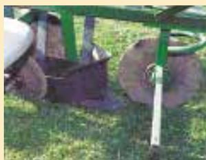
A no-till wavy coultter cuts ground ahead of a V-shaped opener with a cultivator sweep on front.
