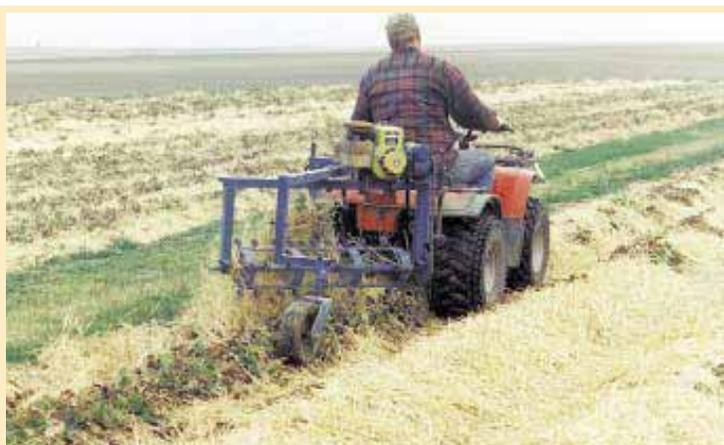
One-row mulch remover works like a side delivery rake to pull straw mulch off strawberry plants at the end of winter. Conrady pulls the machine with a 4-wheeler ATV.
