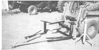
Bale spear, pallet forks, 5-ft. boom and drawbar can be used with the skid steer loader
