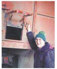
Bauer's homemade latch is equipped with an eccentric that holds end gate tightly in place wherever he wants it.
