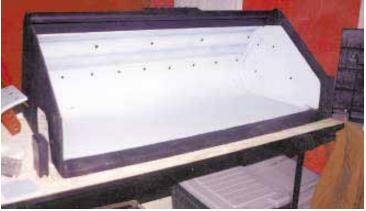
Bolt-on plastic liner comes in sections that are screwed onto the back, sides, and bottom of bucket and then "welded" together at the joints.
