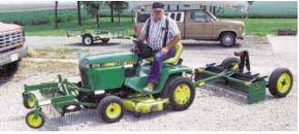
Schlossler mounts a homemade, spring-toothed dethatcher on front of his Deere 318 garden tractor and a box scraper on back.
