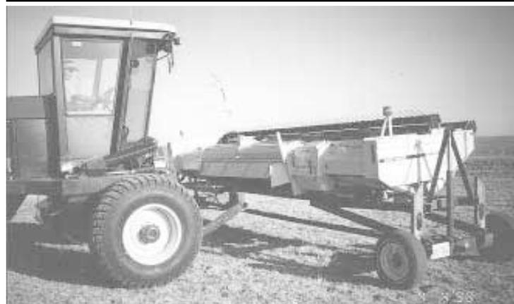
**Cart raises up to 24 in. with a pair of 2 in. cylinders to make loading header easy.**
