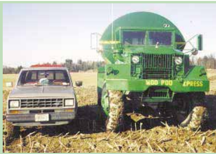
The truck rides on tires that stand more than 4 ft. high and require only 55 psi of air.
