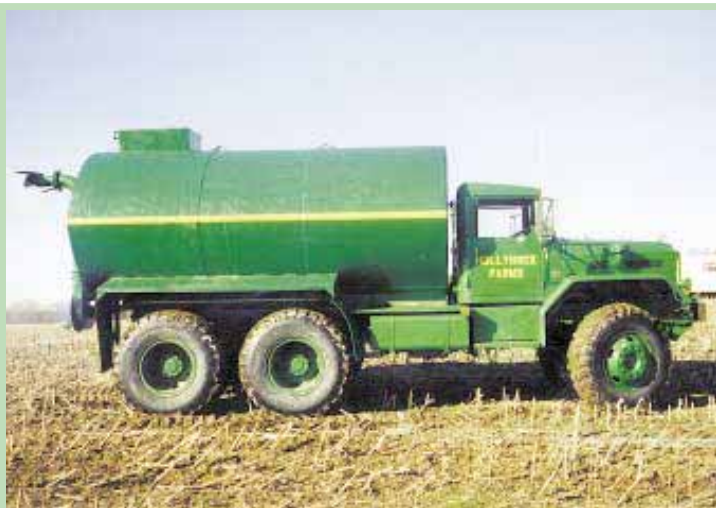
The Kellers equipped the tandem axle truck with a 5,000-gal. liquid manure tank.
