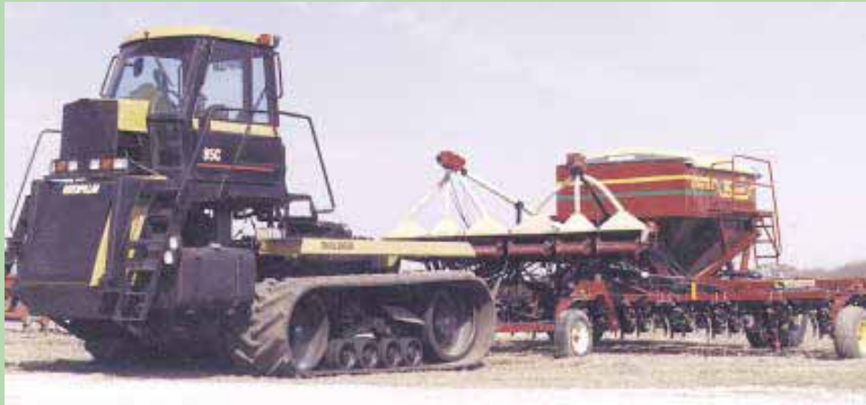
Tim Scheetz rebuilt a 1995 Cat Challenger to pull his Seed Hawk planter. He remounted the cab further ahead on the frame and raised it 16 in. A sliding fifth wheel hitch is used to pull the planter, which is fitted with a detachable "gooseneck" hitch (not shown in photo).
