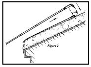
Roof cleaner has a head like a big cheese slicer fitted with a piece of plastic to remove ice and snow quickly and easily. You can push it upward (above left) and snow will slide down plastic sheet that trails behind. Or you can pull downward (above and below) and plastic sheet will come down from above.
