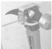
Device fits over the hammer head and is held in place with a nylon strap.
