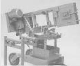
The two-wheeled Ellis 1600 is equipped with a 1-in. wide blade and is powered by a 1 hp, 110-volt electric motor. The turntable mounts on a half-moon casting. A built-in protractor allows for fast and accurate selection of angles, and a movable guide arm can be used to make the cut as accurate as possible.
