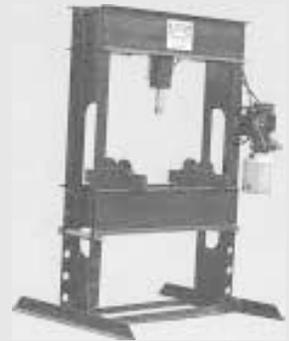
and 2-in. bed pins with hardened holes. It uses single phase electricity; 3-phase is optional. The 100-ton model is 86 in. high and 64 in. wide and has a maximum working width of 48 in.
