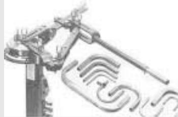
Weighing only 60 lbs. and standing just 38 1/2-in. high, the "Compact Bender" has the capacity to bend up to 5/16 by 2-in. flat steel, 5/8-in. solid round or solid square hot rolled mild steel. A sharp right angle bend attachment (included) bends up to 3/16 by 2-in. or 1/4 by 1 1/4-in. flats.
