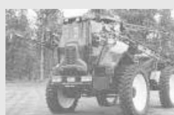
It's powered by a 230 hp Cummins diesel and a Deere-Funk 4x4 powershift transmission. It converts to a spreader using a belt-driven 8-ton fertilizer/10-ton lime spreader. The sprayer offers a 1,150-gal. tank and 60-ft. fold-over boom.
