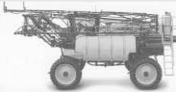
Features: Cummins engine; 60-ft. hydraulic-fold, front-mount boom.
