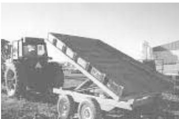
Trailer's tandem axle follow the ground contour and keep the wagon from sinking into soft ground.
