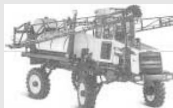
The Ranger series features a 175 hp engine, 80 or 90-ft. boom, and 600-gal. tank.
