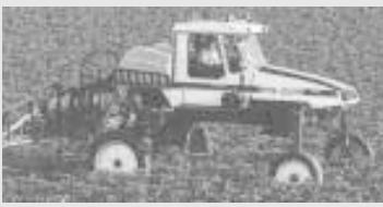
Features: 60-ft. booms; 300 and 400-gal. tanks and 3-speed automatic transmission depending on which model you choose.
