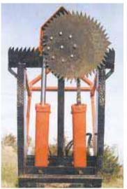
Toothed saw blade is attached to a pair of hydraulic cylinders that rotate blade into tree. Half the teeth on blade point in one direction and the other half point in the opposite direction.
