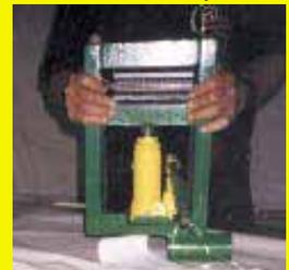
a heavy-duty steel frame. The jack, which fits on the jack stand on the baler hitch, moves a center bar holding a commercial belt lacer up and down. When the jack is pumped up, it pushes the teeth of the lacer into the broken or damaged belt, repairing it on the spot.
