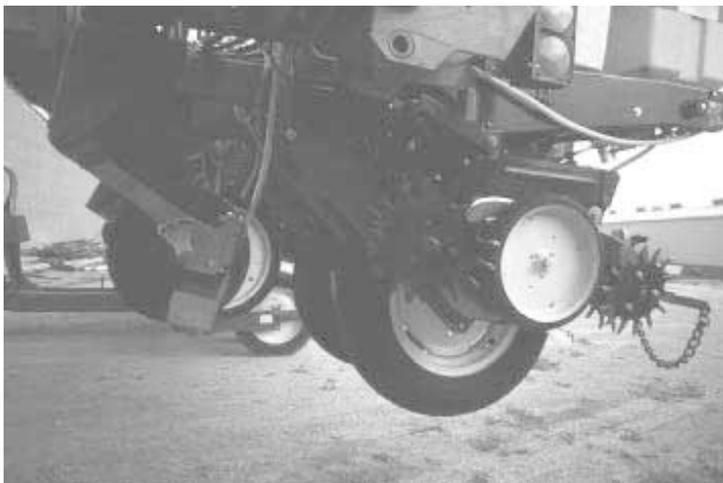
The Reeds' row unit setup includes Deere fertilizer coulters followed by Yetter fertilizer knives, row cleaning wheels, gauge wheels equipped with Case-IH rubber, Martin spader wheels, and a drag chain.
