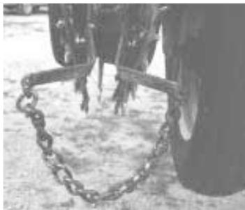
Martin spader wheels and drag chain. The wheels run shallow enough to stay over the seed but still break up any compaction the openers may have left in the seed furrow sidewalls.
