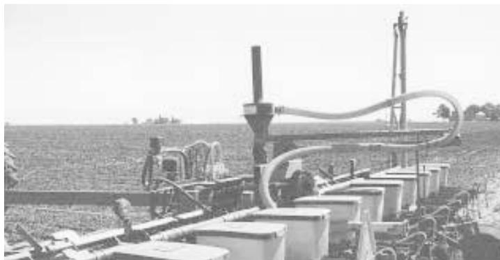
Broaddus mounted a “swing arm” on the planter that's equipped with a cone-type decelerator. It swings across the full width of planter, making it easy to fill.
