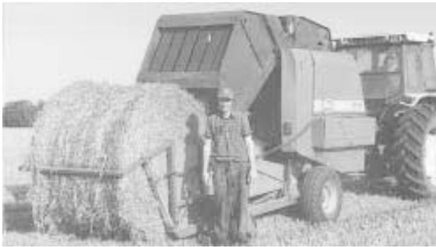
The accumulator attaches to the bale chamber just behind the axle and is designed to group in pairs bales measuring up to 4 by 6-ft.
