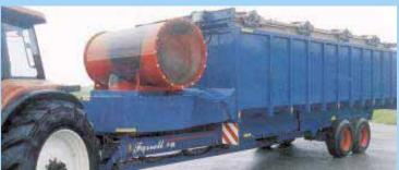
Fan sucks hot air through a large opening under the burner, then forces it through the trailer's perforated drying floor.
