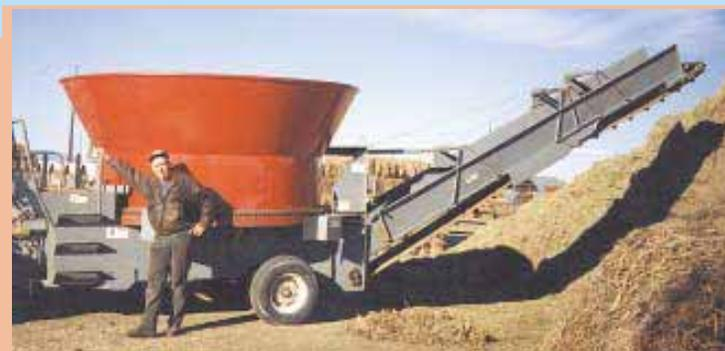
**Tub grinder breaks stems without turning leaves into dust, says inventor Bob Anderson. Pto-driven machine works much like the cylinder and concave inside a combine.**
