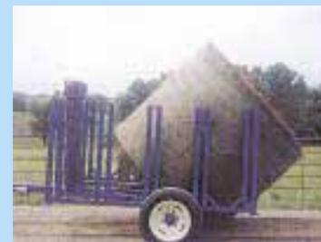
**A winch is used to pull the bale onto the trailer, rotating it 90 degrees.**
