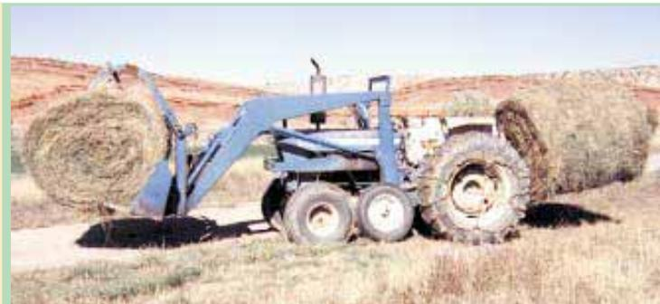
**Roden replaced the original 7.50 by 18 tires (shown here standing between tractor's front and rear wheels) with 11.00 by 16 ones mounted on heavy duty offset wheel rims.**
