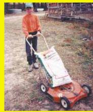
Nine-year-old Chet Logan removed the motor from an old lawn mower so he could haul buckets or bags on top of the deck.
