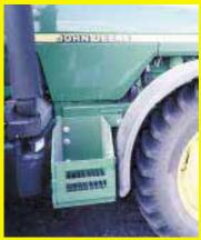
Rock box mounts behind the right front tire and ahead of the fuel tank where it's out of the way. Comes with a spring-loaded latched gate that makes it easy to unload.
