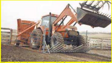
When pushed by a bumper or tires, gate folds flat to ground. Spring-loaded cables attached to corners raise gate back up after vehicle has passed.
